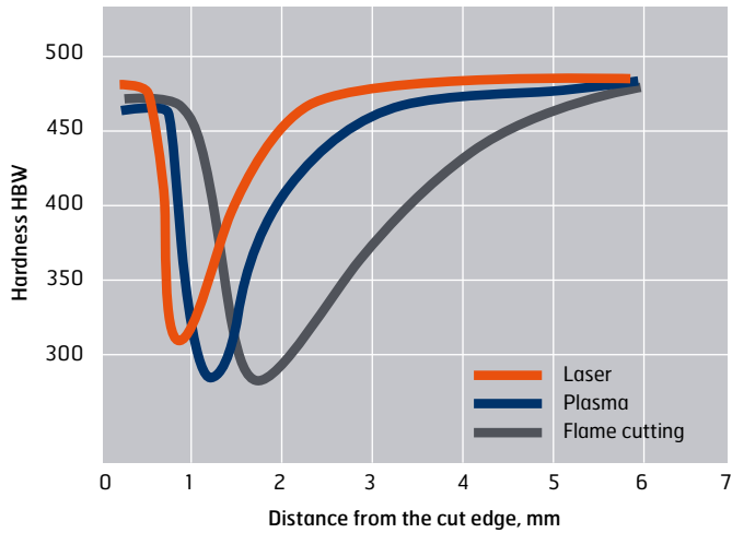
FIGURE 11. ABRASION RESISTANT STEEL PLATE, 6 mm. TYPICAL HARDNESS PROFILE OF A THERMALLY CUT SURFACE ILLUSTRATED FROM THE CUT EDGE TOWARDS THE BASE STEEL.
